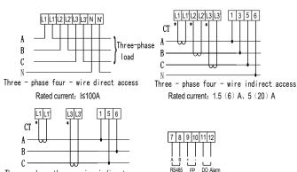
Three - phase three - wire indirect access Rated current: 1.5 (6) A, 5 (20) A
