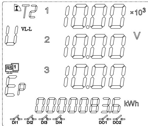
**Note:** in the high voltage measurement, X10<sup>3</sup> mean the showing voltage value multiplied by 1000, in the screen diagram mean the voltage is 10X1,000=10,000volt
