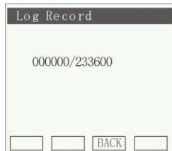
BJ-194Q optional equipped 128M large-capacity memory for storing electrical parameter. Logging secondary side voltage, current, active, reactive power, power factor, frequency value. Total record 233,600\* logging data.
