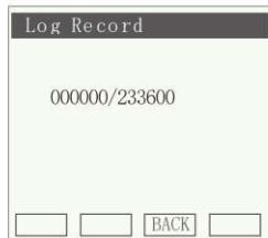
BJ-194Q optional equipped 128M large-capacity memory for storing electrical parameter. Logging secondary side voltage, current, active, reactive power, power factor, frequency value. Total record 233,600\* logging data.
