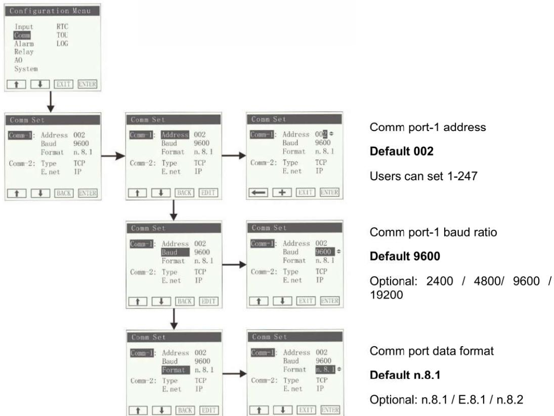
**Note:** 194Q optional dual communication port; Comm-2 can be used for external HMI or other special operation, default only Comm-1 is valid.
