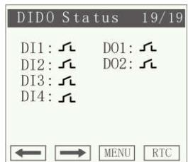
BJ-194Q optional max 6\*DI port, uses dry contact resistance switching (passive node), with +15V meter internal power supply, for detecting variety of outside coil status.
