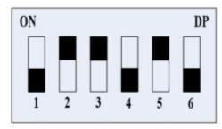
Alarm resistance threshold is  $600 \mathrm{K}\Omega$
