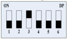
Alarm resistance threshold is  $20 \mathrm{K}\Omega$
