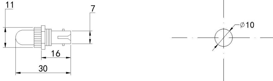
Arc light sensor external shape and hole size (Unit: mm)
